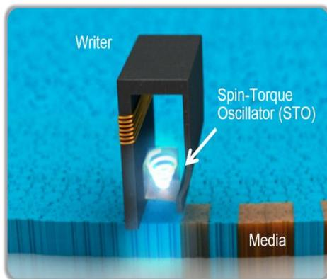
*In a MAMR drive, the spin-torque oscillator (STO) generates a microwave field to provide assistance when magnetizing the grains prior to a write*
