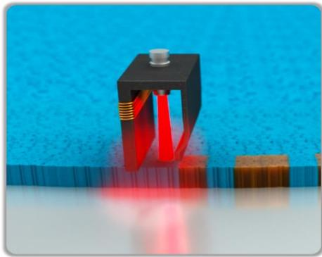
*In a HAMR drive, a laser diode heats the media to assist in magnetization*
