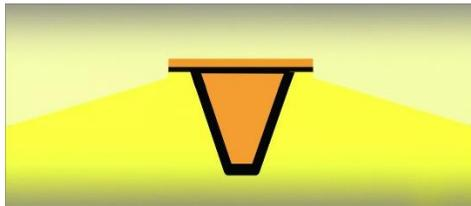
*Tapered write head using the Damascene process*
