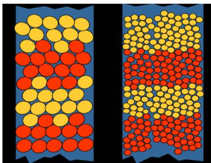
*Each bit is stored in magnetic grains within continuous magnetic film -- Increasing disk capacity requires smaller grains on the media, and a smaller head to magnetize the grains*
