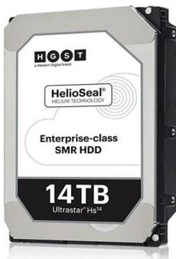
Western Digital's HGST-branded Ultrastar®Hs14 helium-sealed HDD
